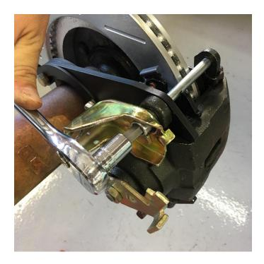
The calipers can now be installed using medium strength threadlocker (such as Loctite 243) on the two 7/16-20 caliper bolts and torque to **30 ft-lbs**. **NOTE:** If there is too much pressure on the outside pad once installed, remove the spacer between the axle flange and caliper bracket. **For parking brake calipers, refer to the instructions below for Parking Brake Caliper Setup.**
