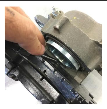
**Kits with non-parking brake calipers** should be checked to confirm the machined pad spacers are present and make sure the notch in the pad spacer lines up with the corresponding boss on the brake pad.
