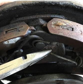
Remove the additional retaining springs from the brake shoes.
