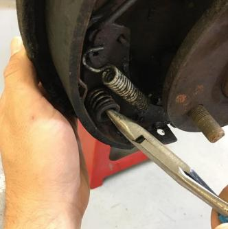
This installation refers to the **passenger side** of the axle. All steps are to be repeated on the driver side. Start by removing the factory drum. It may be necessary use a lubricant around the axle register to do this. Once the drum is removed, remove the brake shoe retaining springs (2 places) as shown.
