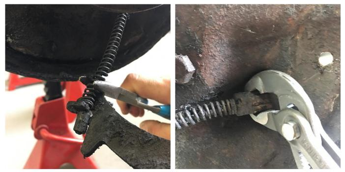
Disconnect the parking brake cable from the brake shoe, then remove and discard the brake shoes and hardware. The cable can then be removed from the backing plate by depressing its perimeter springs.
